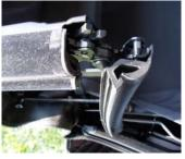
rubber surface on the left has fuzz (flock) on it - so NO grease is used on this rubber to rubber contact. You might also notice a U shaped metal piece on the left and a corresponding pin that it locks to on the right - this should get a very thin coating of the lithium grease. The pivot point for the U shaped piece should get a drop of the motor oil. Three different lubrication challenges in the space of about 2"
