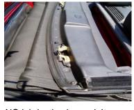
this track has fuzz on it - so NO lubrication is used. It helps keep it quiet if the track is clean and polished. I wax mine with Zaino when I do the car. On the E36 - the rubber seal that sits here is not flocked, and is a primary cause of NOISE and squeaks if it isn't kept lubricated. I used to lube this seal using the rubber pad on the GummiPhlege tube. A thin but noticeable coating is good.
