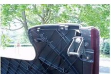
thin coating of the silicone grease. At the top center - you see the rubber seal for the front edge of the tonneau cover to the inside of the car - on the E46 this has fuzz - so no lube necessary. On the E36 (from memory) - it is bare rubber - so some silicone lube is a GOOD thing. You
